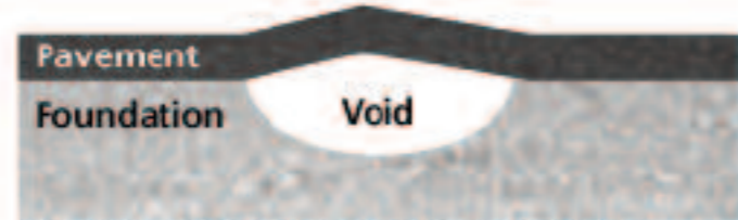
The ground thaws and leaves a void in the foundation.
