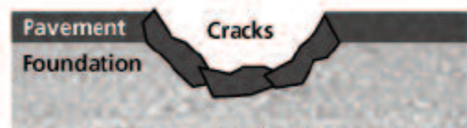
Unsupported pavement fails under the traffic load.
