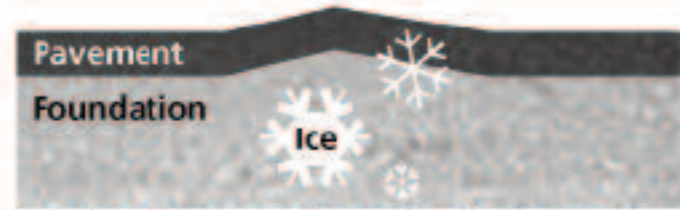
Freezing water expands causing displacement of the pavement and/or foundation.
